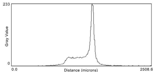
FIG. 1. Vertical cross section through the collimated beam 2.4 m behind the multiprism.
