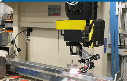
L-bend Vacuum Chamber Welds
