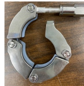
Quick-Seal ConFlat Chain Clamps from VACOM 1040 of 1920 delivered
