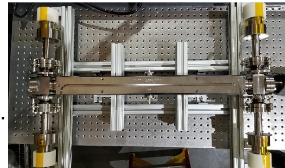
First assembled high-voltage stripline injection kicker at BNL
