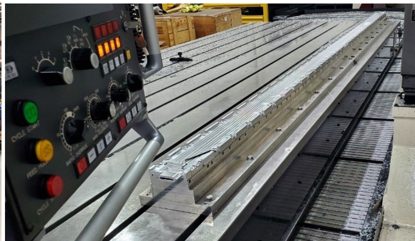
Cold vacuum chamber being machined for 2 nd SCU
