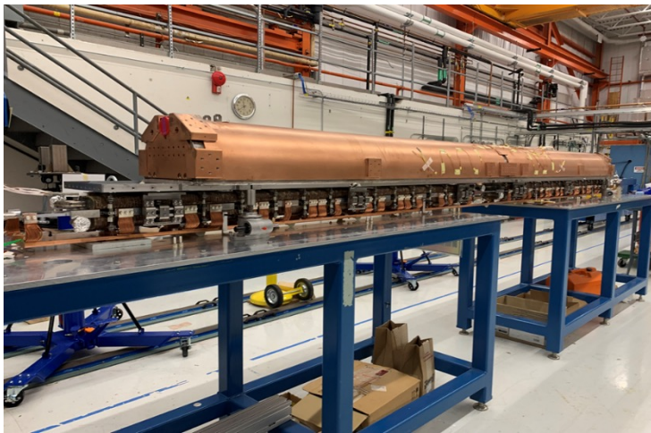
Cold mass with LHe tank, two sets of magnets and beam chamber for 1 st SCU
