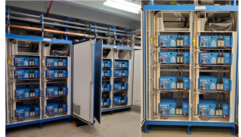
Unipolar power supply converter cabinets and the units under test in elevated-temperature room.
