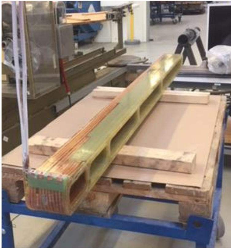
Epoxy impregnated M1 coil
