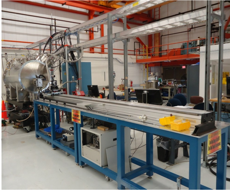
Figure 3.5-30: View of 3.5-meter linear stage on the upstream end of the SCU0 cryostat.
