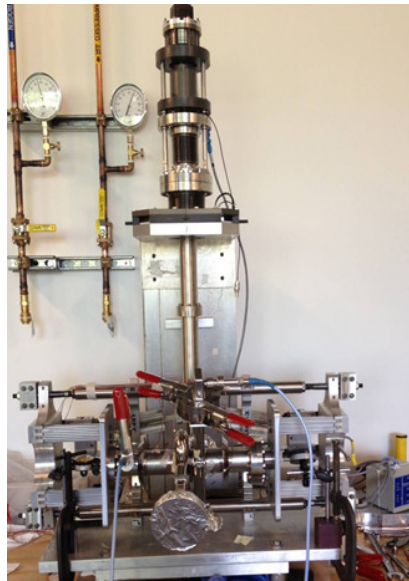
Figure 3.6-143: Cavity CCA3-1 being measured in CEBAF C100 tuner test stand.
