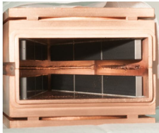
Figure 3.6-152: Full HOM damper without rf flange.
