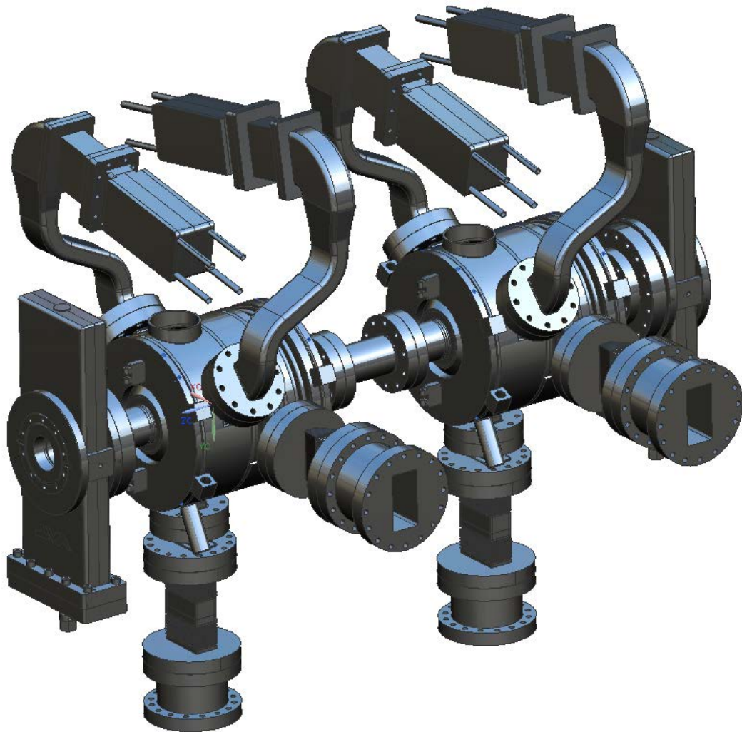
Figure 3.6-97: SPX0 2-cavity assembly.
