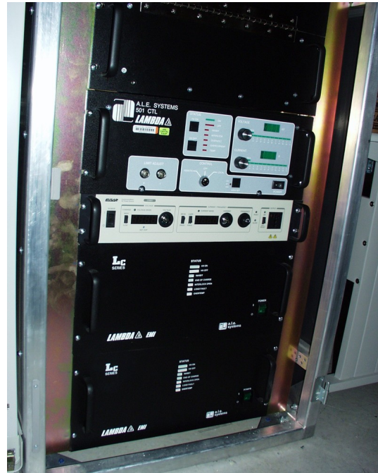
Figure 3.6-120: Photo of TDK-Lambda high voltage power supply used to supply beam power for the SPX-0 klystrons.
