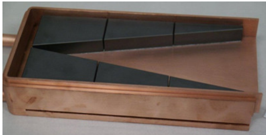
Figure 3.6-151: Half of a prototype HOM damper prior to electron-beam welding.
