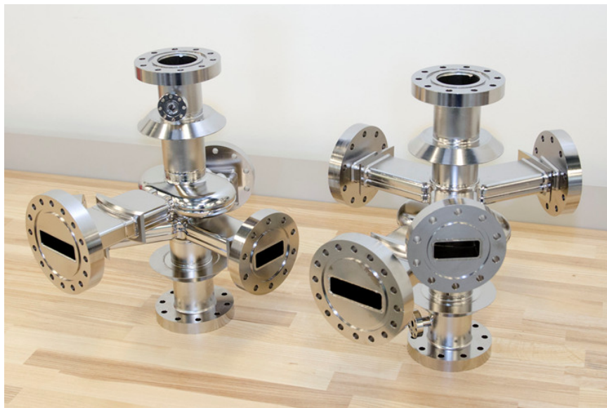
Figure 3.6-141: Two of the three SPX0 cavities fabricated at JLab.
