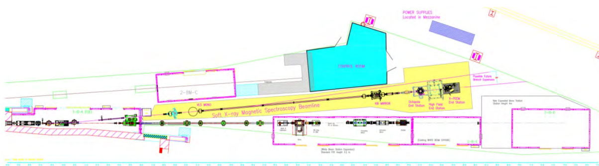
Figure 4-116: General layout of the soft x-ray magnetic spectroscopy beamline in the 2-ID location being considered. Space requirements around beamline optics and experimental stations are highlighted in yellow. Approximate size and location for a control room is also shown.
