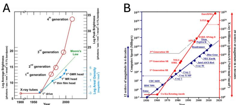
Figure 1-16 Data and compute needs are outpacing traditional computer scaling. Brightness of facilities over the last 60 years is plotted against Moore's law A) and the evolution of the fastest supercomputer in the world B).
