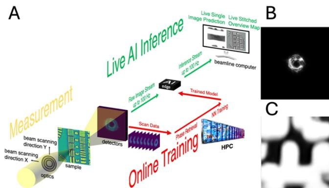
Figure 1-17 HPC + AI@Edge enables real-time, streaming ptychography. A) Schematic of workflow moving data from instrument to Polaris for labeled data generation and training. The trained model is pushed to the edge for live inference. B) Detector image that is input to the trained network. C) Single-shot prediction from the network.
