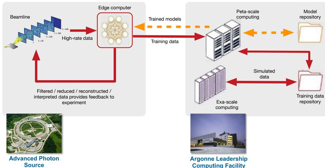
Figure 1-14 Edge computing architecture using machine-learning models trained on supercomputers.
