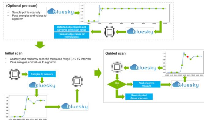
Figure 1-6 Optimized XANES scan enabled via Bayesian optimization and Bluesky Adaptive. Contact: Ming Du.
