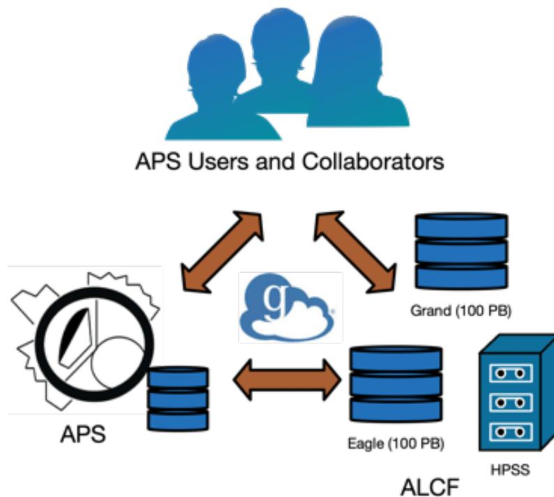
Figure 1-9 Storage available for APS beamlines. A multi-PB data storage system located at the APS serves medium-term needs. The ALCF provides multiple systems for long-term storage. Capacity will be expanded as needed to meet sponsor requirements.
