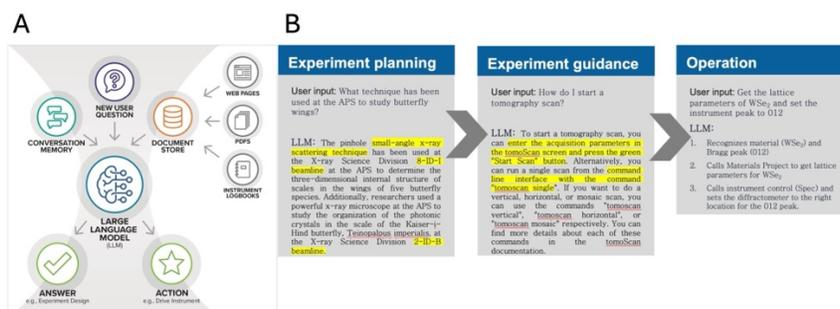
Figure 1-19 A) Overview of CALMS: CALMS uses a large language model in conjunction with conversational memory, document stores, and experimental tools to answer user queries or take action to drive an instrument. B) Examples of CALMS interacting with a user in the experiment planning stage, guiding an user through data acquisition and directly calling instrument controls with user input.
