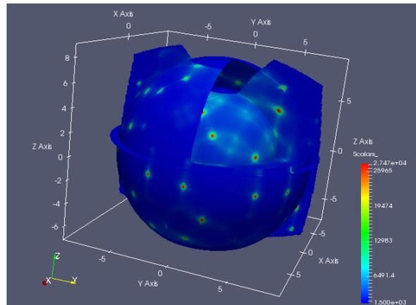
Figure 2-5 Visualization of a dataset from a pixel from a Silicon analyzer crystal processed with RSMaP3D. This data shows a combination of diffraction (bright spots) and thermal diffuse scattering (broad lines connecting diffraction spots). This data was taken on the High Energy Resolution Inelastic X-Ray Spectrometer (HERIX) at APS Sector 30.
