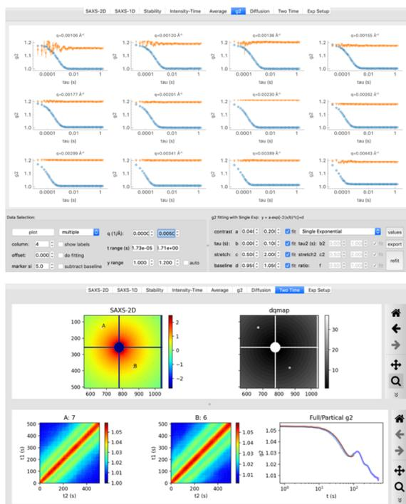
Figure 2-8 Top:  $g_2$  plots of the multi- $\tau$  correlation results. Users have many options to visualize data. Bottom: Visualization of a two-time correlation of a rubber sample. Users can select the region of interest by clicking the mouse.
