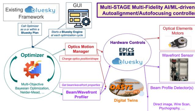
Figure 1-5 Schematic of Oasis digital twin integrated with a beamline via Bluesky and its Bluesky Adaptive framework. First tests are imminent at Sectors 8-ID and 25-ID. See L. Rebuffi, S. Kandel et al., Opt. Express **31**, 39514 (2023). DOI: 10.1364/OE.505289.
