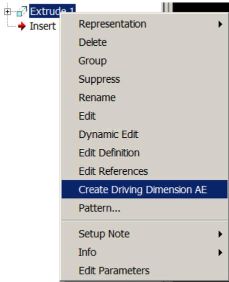
5. Read the message: One or more dimensions were not converted to driving dimension annotation element, because the extruded distance is along the z-axis. Add it in when dimensioning the top or right view.
