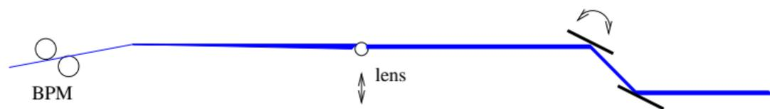
runs a program in the MOSTAB to control the monochromator piezo and moves the lens to keep the monochromator tuned up
