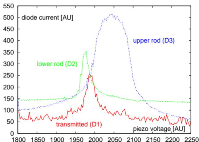
scan piezo (DAC output), acquire 3 signals on ADC inputs (D1 .. D3)
