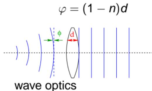
weak refraction  $\rightarrow$  many ( $N$ ) lenses (compound refractive lens)
