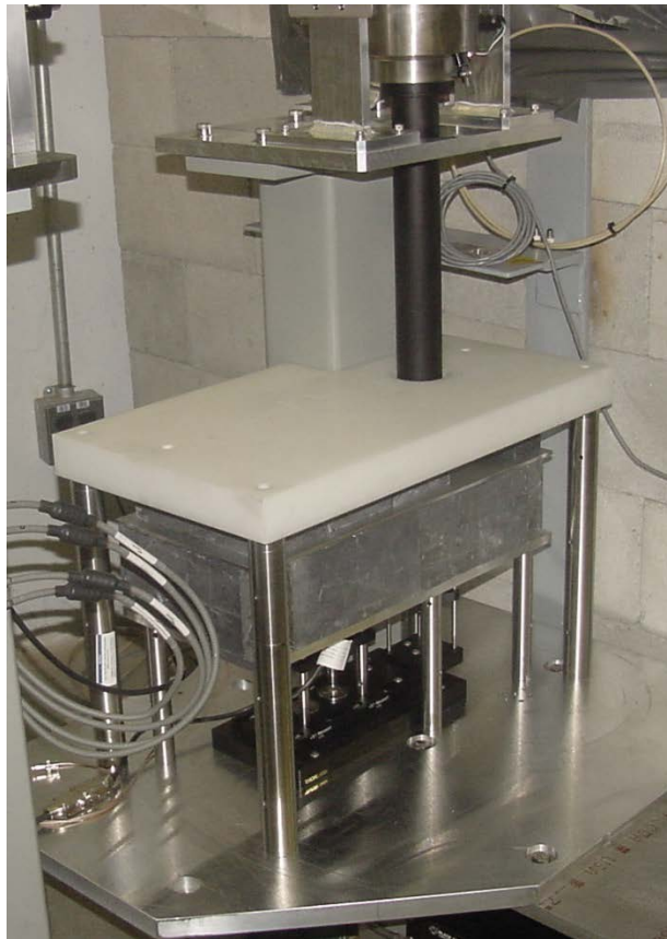
Booster beam dump (BTX) Transverse Profile Monitor prototype imaging hardware located under the electron beam vacuum pipe just upstream of the dump shielding wall.
