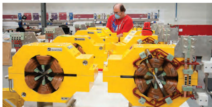
Technician Senior Bob Furst (APS Engineering Support Division Mechanical Operations and Maintenance Group) at the APS-U Magnetic Measurement Laboratory in Bldg. 369, testing the pole tips on sextupole magnets for the APS Upgrade multi-bend achromat storage ring.
