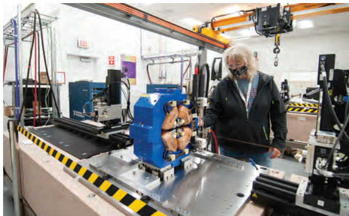
Kris Mietsner (APS Engineering Support Division Survey and Alignment Group) at the APS-U Magnetic Measurement Laboratory in Bldg. 369, collecting data from an APS-U storage ring quadrupole magnet for analysis – this is called fiducializing the magnet. These data are used for aligning magnets to each other in a module assembly.
