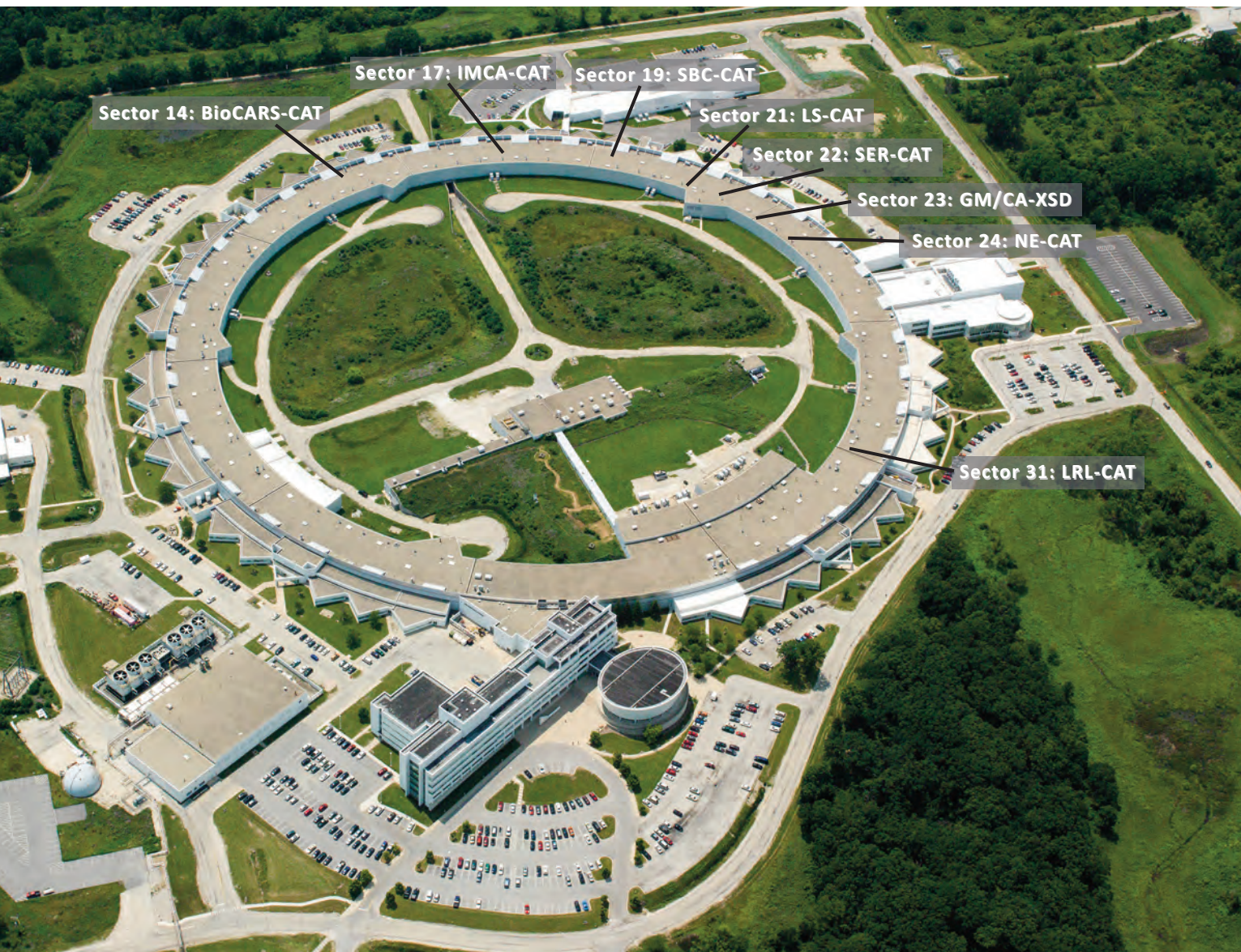
The APS facility at Argonne National Laboratory. Sectors comprise one or more x-ray beamlines. Locations of the macromolecular x-ray crystallography sectors (see facing page) are indicated in the photo above.
