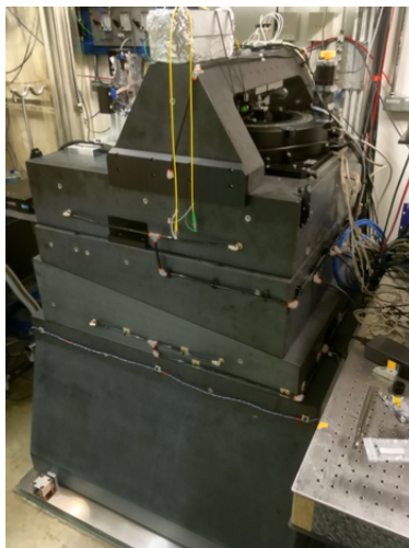
Figure 6.15. The Velociprobe instrument at APS with stable granite components capable of micrometer reproducible movements.
