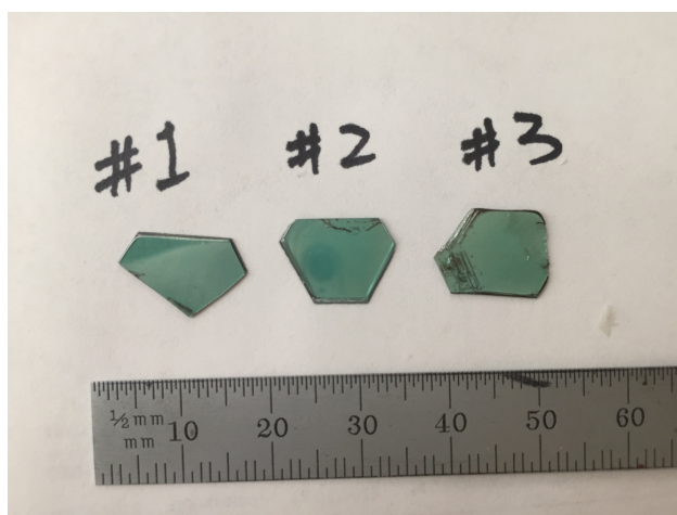
Figure 6.90. Three single crystals of 6H-SiC used in white beam topography and mono beam double crystal rocking curve topography [18].
