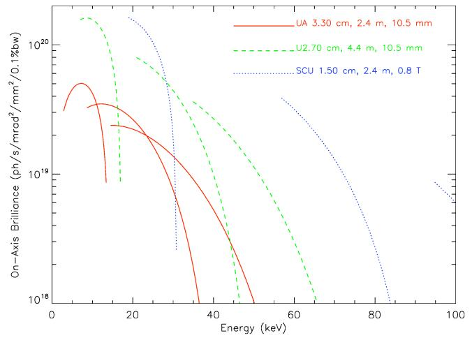
Superconducting undulator surpasses Undulator A ~ 10 times at 25 keV (when magnetic field errors are taken into account)
