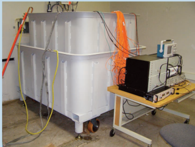
150-kV Marx high-voltage pulse generator
