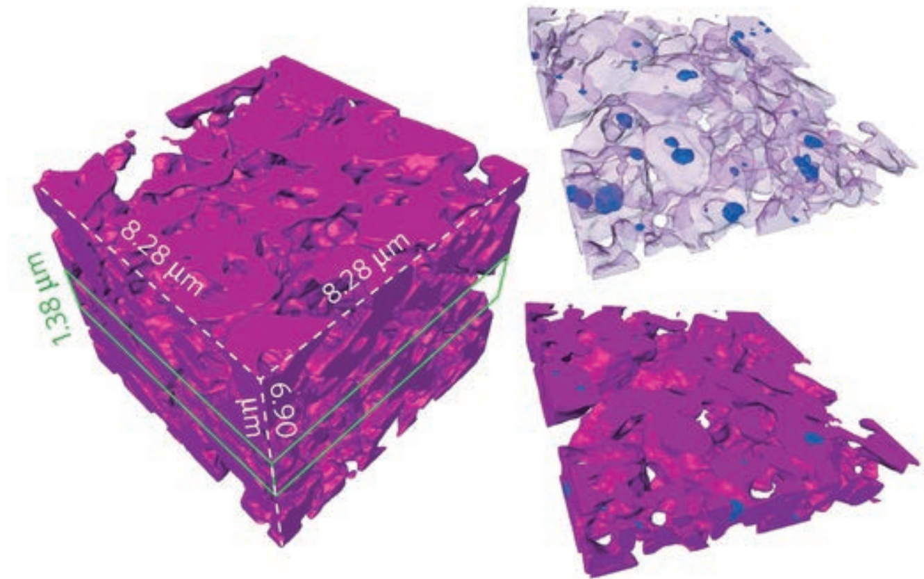
Fig. 1. Transmission x-ray microscopy three-dimensional data set of a representative region of mesostructured silicon (left). A thin slice of the data set (green lines) highlights the presence of both intra- and inter-granular voids (right). Representing silicon as a semi-transparent matrix allows clearer visualization of the voids (upper right). Magenta, silicon; blue, intra-granular voids; open regions in the whole volume or thin slice, inter-granular voids.
