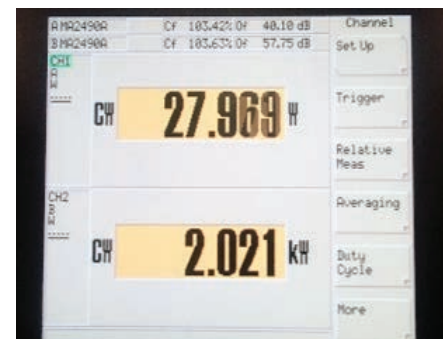
Fig. 3. Rf power meter indication from first operation at design goal of 2-kW cw rf output.
