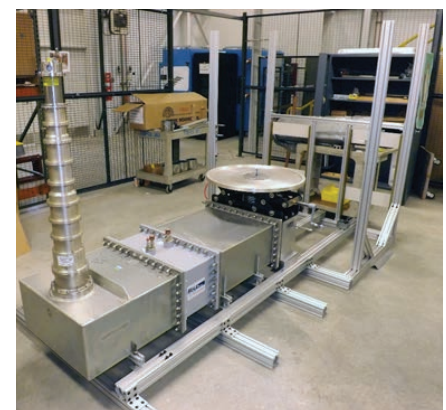
Fig. 5. Assembly of 12-kW demonstration system, showing the base of the output-combining cavity assembled to the waveguide line and terminating load.
