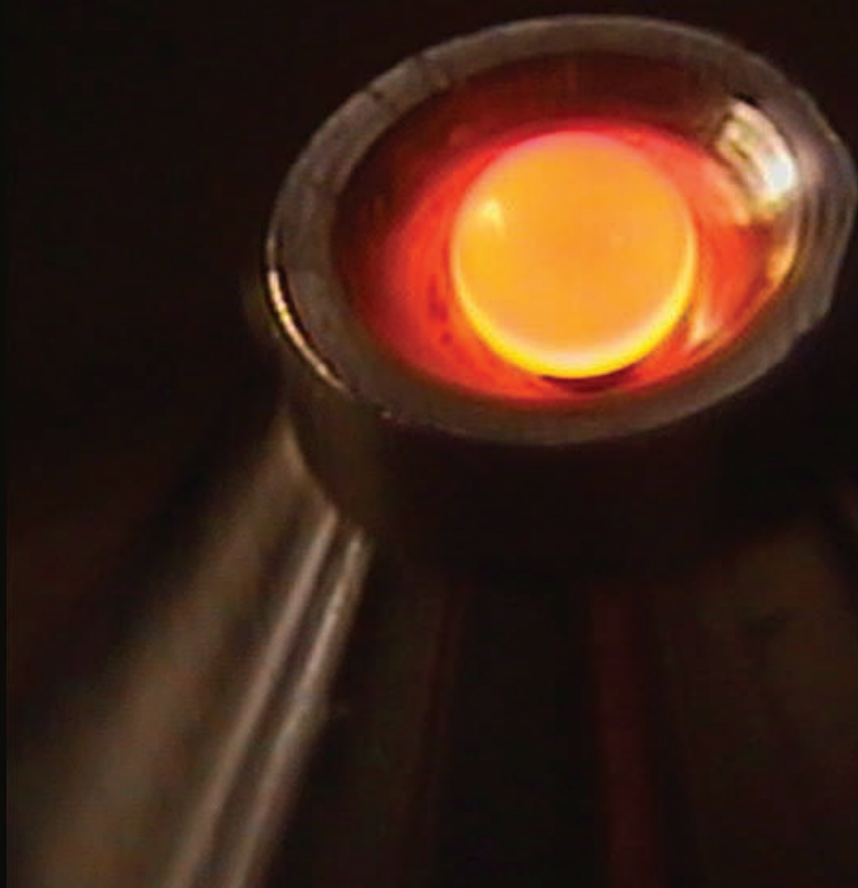
Fig. 1. A spherical bead of borate suspended in an aerodynamic levitation furnace.
