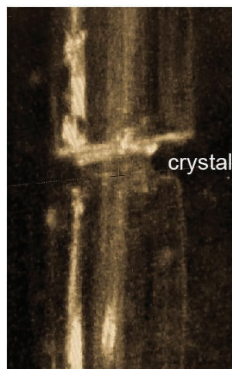
Fig. 1. Image of the custom-made EF-X crystallography set-up. The left panel shows how the apparatus that holds the crystal and applies the electric field pulse (red arrow) is positioned relative to the x-ray beam (white arrow). The right panel shows a close-up of the protein crystal held between two glass capillaries that serve as electrodes. The crystal is glued to the bottom electrode while the electric field pulse is transmitted through the top electrode.
