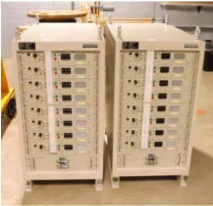
Figure 2. (Left) The first prototype 32 kW prototype solid-state amplifier received from R&K. (Right) The concept for a 200-kW amplifier. Each rack contains 15 2-kW amplifiers that are combined in the combiner cavity hidden below the waveguide. The first prototype amplifier will be tested on the combiner cavity later in 2019.
