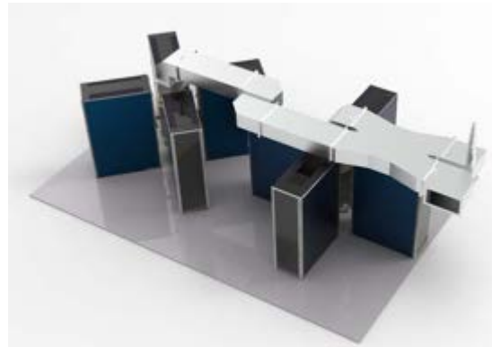
Figure 2. (Left) The first prototype 32 kW prototype solid-state amplifier received from R&K. (Right) The concept for a 200-kW amplifier. Each rack contains 15 2-kW amplifiers that are combined in the combiner cavity hidden below the waveguide. The first prototype amplifier will be tested on the combiner cavity later in 2019.
