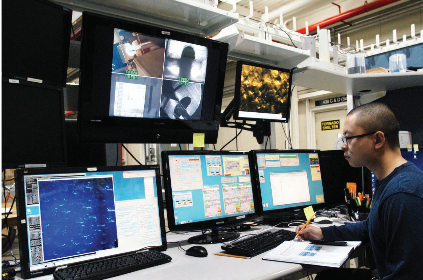
Chen Zhang (Michigan State Univ.) at the 34-ID-E control station, monitoring his experiment utilizing microbeam Laue diffraction to characterize the microstructure beneath the sample surface of a deformed titanium specimen. The information gathered will be the basis for a 3-D computational model that will allow direct comparison between simulation and experimental data. The lower-left screen shows the diffraction pattern being obtained from the sample under study. The control panels in the lower center are to monitor the beam and systematically move the specimen. The top center screen shows real-time video of the measurement from four points of view. The upper right screen shows a birds-eye view of the material area being investigated.
