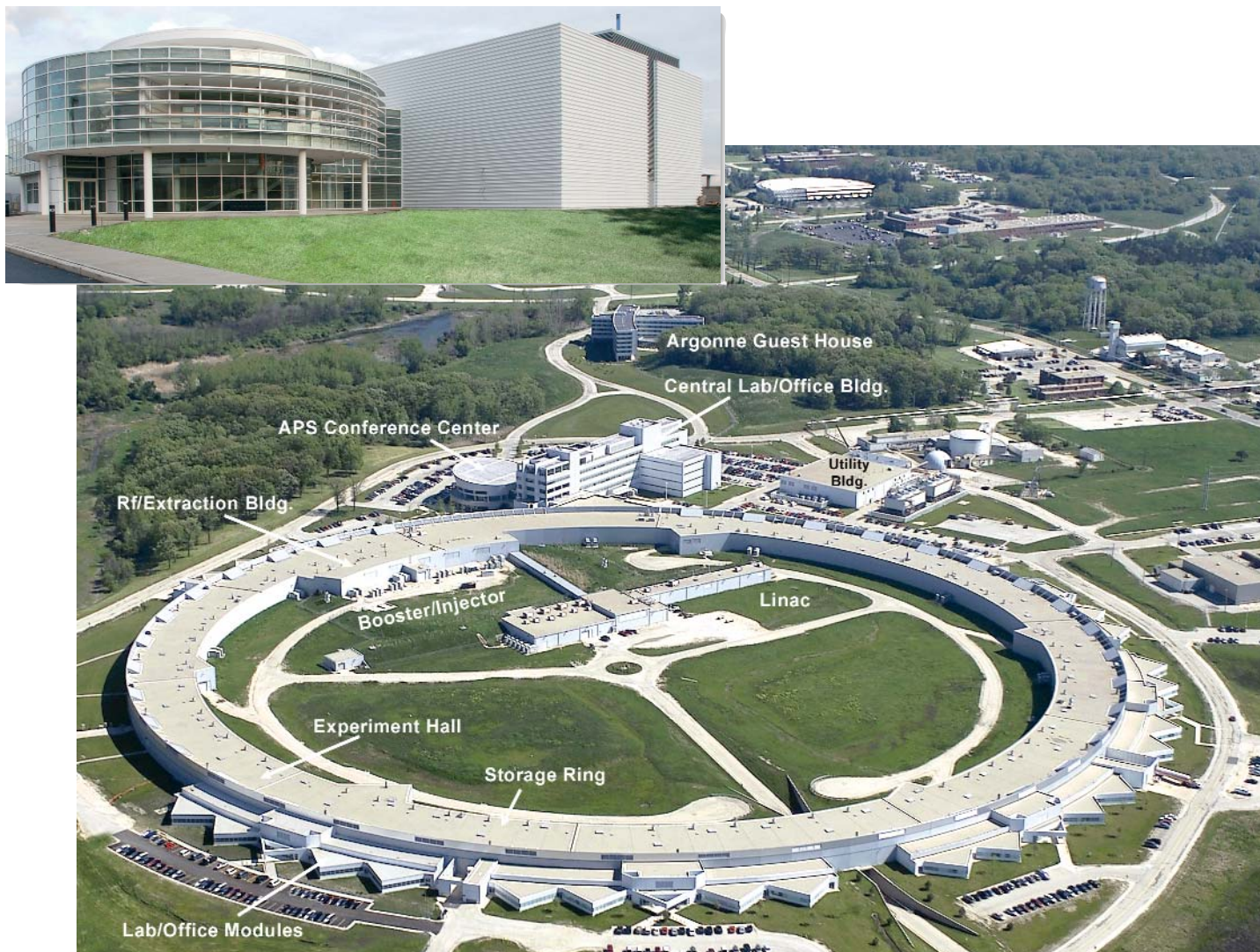
The Advanced Photon Source (APS) facility. Inset: the Center for Nanoscale Materials. The APS occupies an 80-acre site on the Argonne National Laboratory campus, about 25 miles from downtown Chicago, Illinois.
