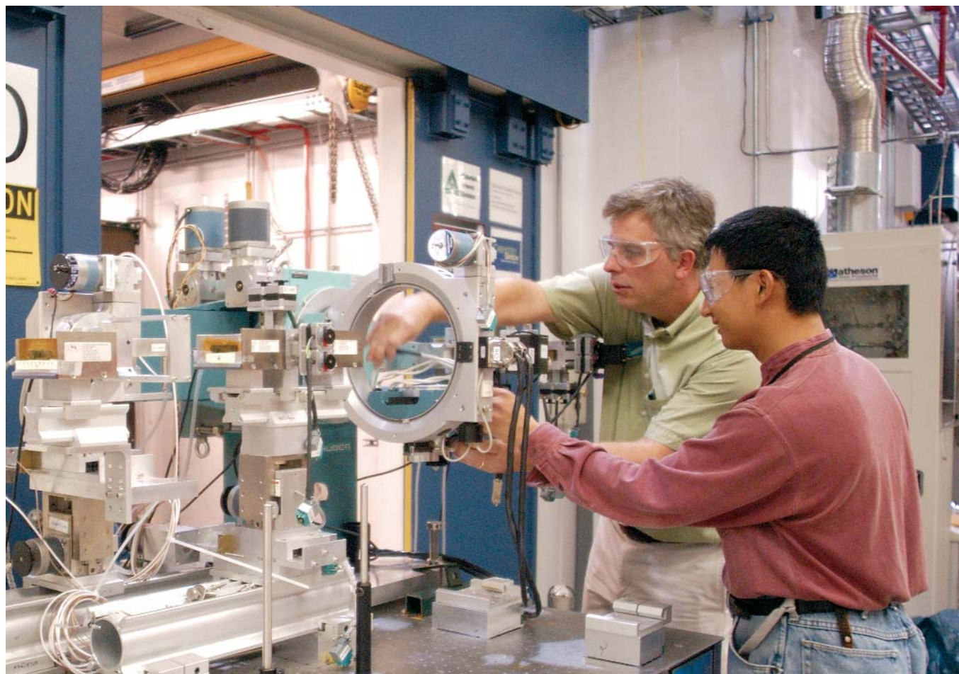
Paul Fenter (left) and Zhan Zhang at the mineral-fluid interface spectrometer on the XOR/BESSRC 12-ID-D beamline.
